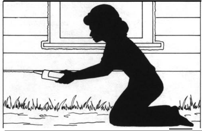
Caulking at the foundation sill is one of the most overlooked yet most important places to stop infiltration.
